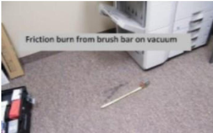
This photo also shows friction burns in carpet, however this time it was caused by the revolving brush bar on the upright vacuum. The vacuum the copier repair person used. He forgot the brush bar continued to revolve when he was using the on-board attachments while vacuuming out the copier.
