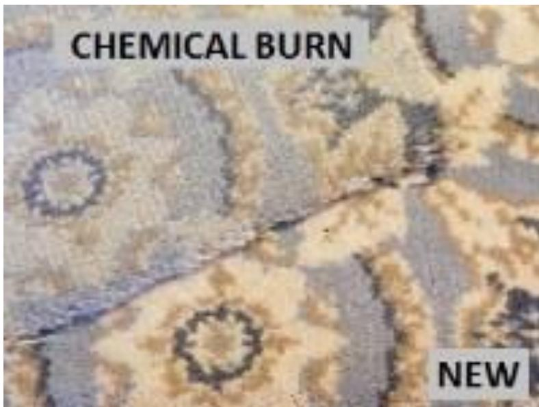
In this photo, it shows carpet made with wool damaged due to improper chemistry. The pH of the chemical the cleaner was repeatedly using was too alkaline. The wool fiber was chemically burned.
