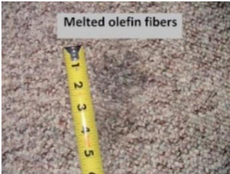
This photo shows the Berber style, olefin/nylon carpet to be melted. I was asked to determine if a certain over-the-counter solvent based spot remover melted the carpet fibers. Ahhh....no. It was the teenager who used a hair dryer to flash dry the carpet before mom got home. Olefin has a very low melting point.
